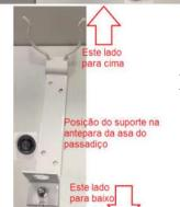
Attach the complete support to the bulkhead of the bridge wing in this position.
